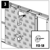
Screw with the fastening kit FIX-SB 45S35. Observe the wall-mounted element manufacturer's recommendation as to spacing.
