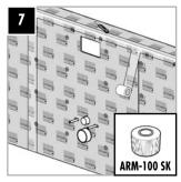
Reinforce all element joints and transitions with glass fibre reinforcement strips ARM-100 SK and . . .
