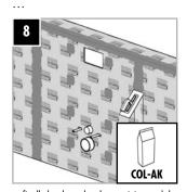
... finally level out the element joints and the heads of the mounting elements with COL-
