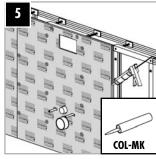
... glued together and glued together with the support construction. Apply the adhesive to the plate edges as an uninterrupted strand.
