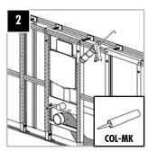
Apply COL-MK on both the support structure as well as on the element. We recommend a snake-shaped application of cartridge adhesives.
