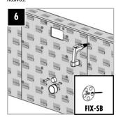
After bonding with the construction and the wall screw tight using FIX-SB 45S35.
